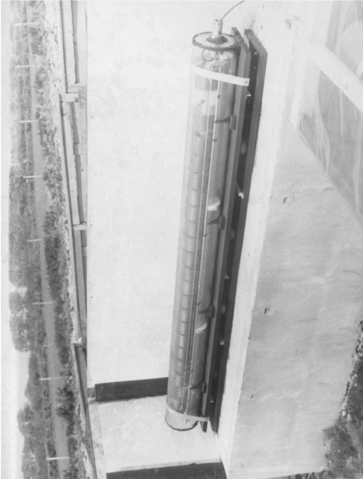
Figure 5 The detector head and coils of one 2m magnetometer in a sealed Perspex tube and lying on its concrete block, showing the anti-vibration mounts (This picture taken in 1965 during the installation of the wind shields and fencing.)
