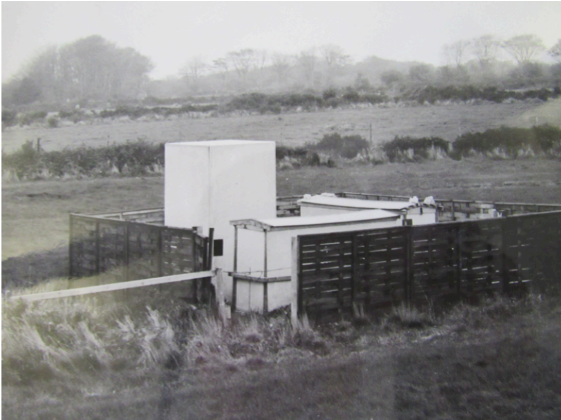
Figure 9 The three-component induction magnetometer system in operation from 1965, with the two horizontal NS and EW units alongside the vertical Z-component added in 1967 in the big white box. Note the windshields and fencing, with the signal cable support being the horizontal wooden strut on the left. There is a complete absence of gorse bushes due to the site being plowed and grassed, and the hedge and field behind are where the induction loop cables were buried.
