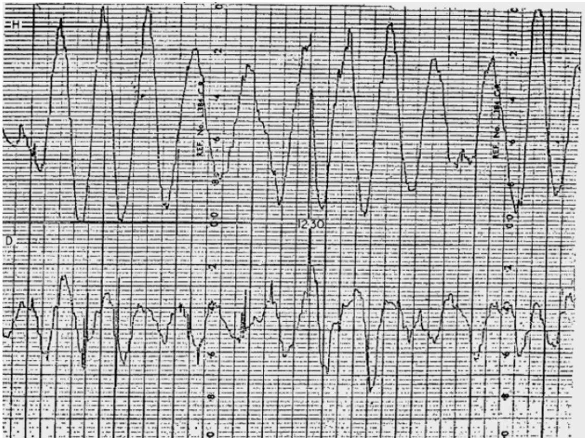
Figure 6 Some typical PC3 micropulsation waveforms that had frequencies centered on about 30MHz and magnitude about 10^{-5} of the main field
